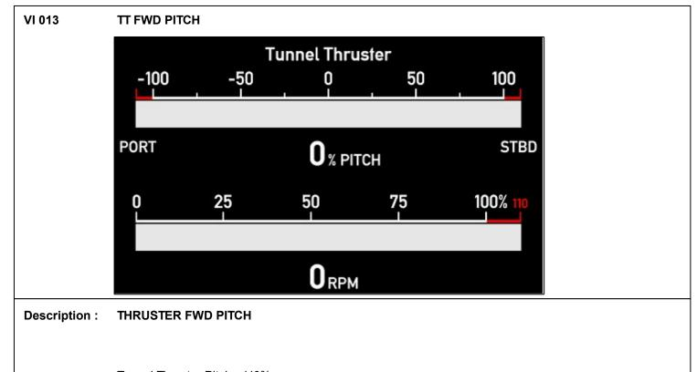
Tunnel Thruster Pitch ±110% Actual Pitch range ±200% with digital readout Tunnel Thruster RPM 0...110% Actual RPM range ±3276 with digital readout
