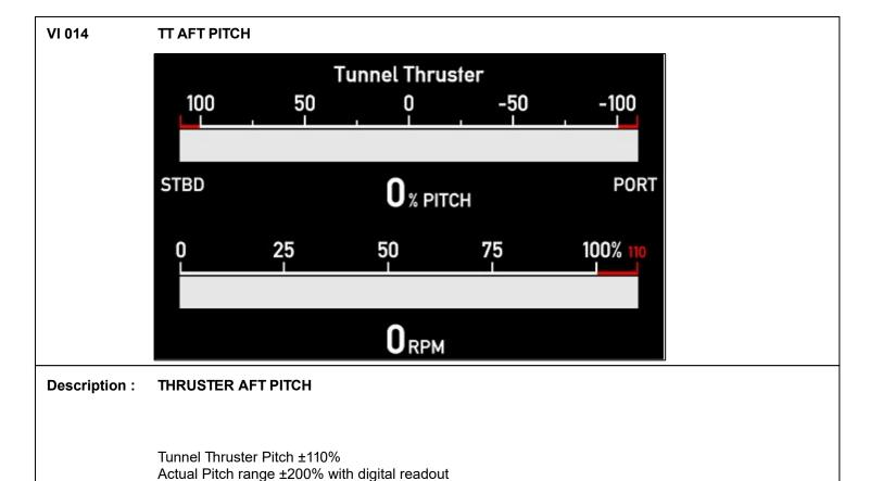
Tunnel Thruster RPM 0...110% Actual RPM range ±3276 with digital readout
