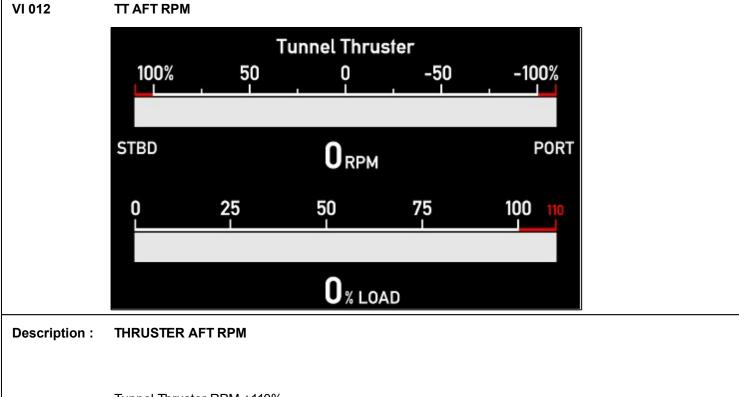
Tunnel Thruster RPM ±110% Actual RPM range ±3276 with digital readout Tunnel Thruster Load 0...110% Actual Load ±200% with digital readout
